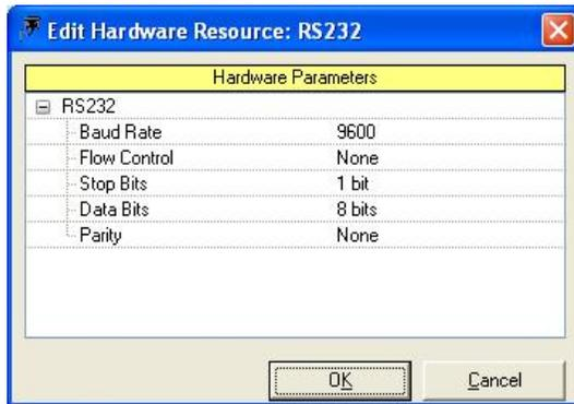
Figure 75: COM Port Configuration (FX Builder Side)
