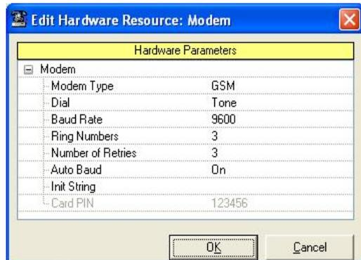
Figure 76: Modem Type Configuration (FX Builder Side)
