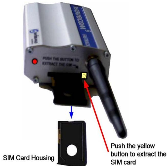
**Figure 26: SIM Card Installation**
